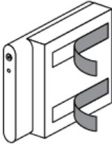
**Note:** Use care when mounting the amplifier and drive packs to the back of the whiteboard. The supplied adhesive is intended to be permanent. If you need to remove or reposition the components, additional supplies are provided. Refer to “Removing and replacing the cable tie holders, driver packs or amplifier”.
