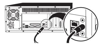
13 Connect the video input cable to the video input port (DB-9), then connect audio and video from a video source to the video input cable. Use either the RCA composite video input or S-video input and either the XLR inputs or RCA inputs.
